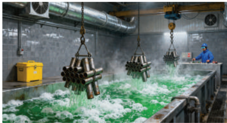
Pickling for rust removal
