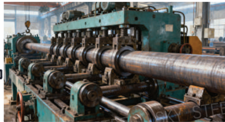
Steel pipe straightening
