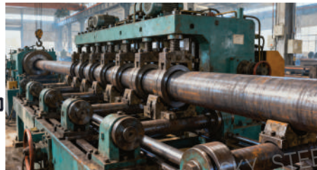
Steel pipe straightening
