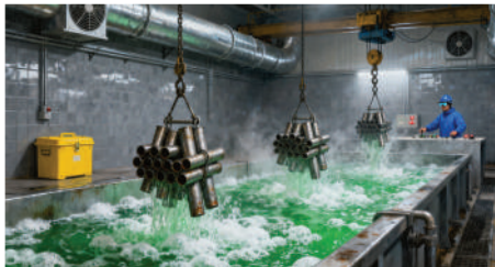
Pickling for rust removal
