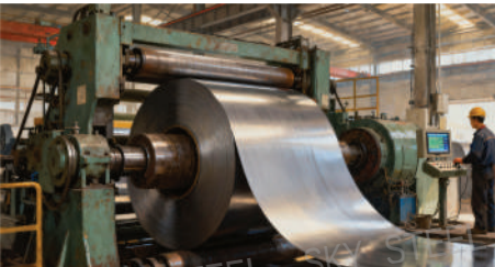
Uncoiling of steel coils
