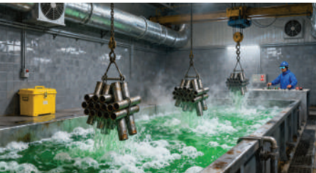
Pickling for rust removal
